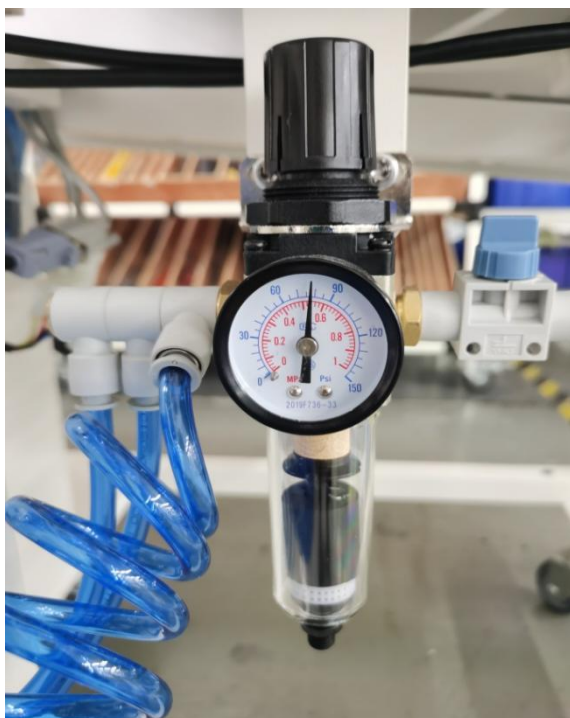
The remaining pneumatic control components are controlled by this pressure gauge, with a factory setting of 0.5 MPa
