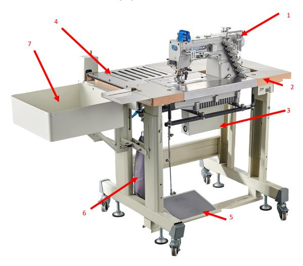
1: BS-FT7010 head; 2: Switch; 3: Control box; 4: Turnover device; 5: Pedal; 6: Suction; 7: Stacker
