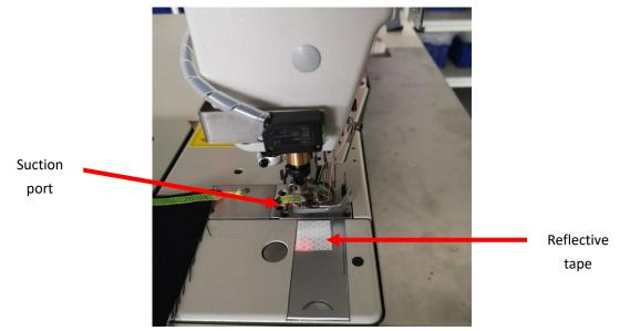
(1) Suction: after starting the machine, step forward on 4.1 - (2) foot pedal to start suction. When the cloth covers the reflective tape, the suction stops after a short delay. When the reflective tape is exposed to the suction, the foot pedal releases to stop suction.
