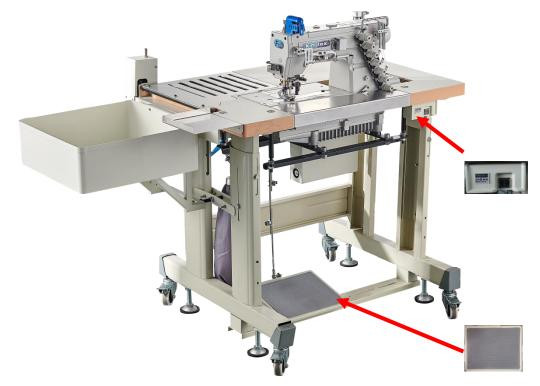
(1) : Power switch: press the power switch to 1, and the equipment is powered on and ventilated.
