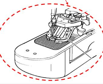
Adjust button clamp position through above red circled M5 screw to be sure needle tip always match button hole center in each single stitch
