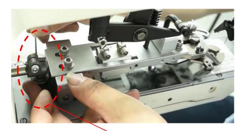
Fix button clamp from backside with screw to be sure smoothly movement up/down, adjust button position after clamp fixing.
