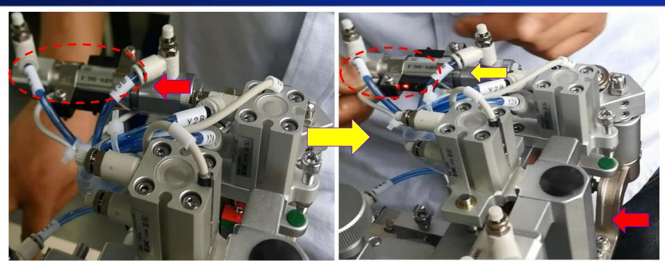
Sensor X5: is to detect if button claw cylinder return back to desired position. sensor X5 light should be ON after button claw controlled cylinder return back, if sensor position not setting properly, Button feeder will not go for next step even button claw reture back.
