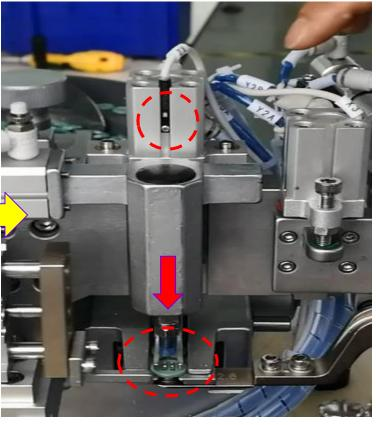
Function of X2: error E01 will come out while there is no button in above red marked position, and machine will stop, in the meanwhile sensor X2 light will be in ON status, while no button.
