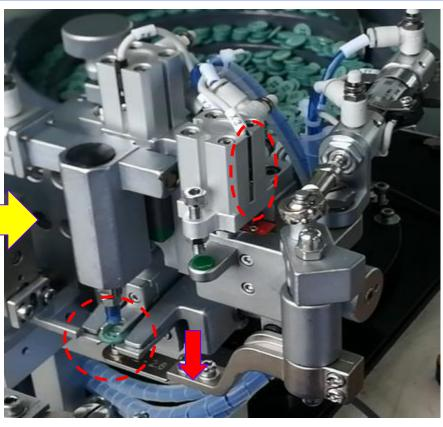
Function of sensor X3: to detect if button claw catch button successfully or not.
