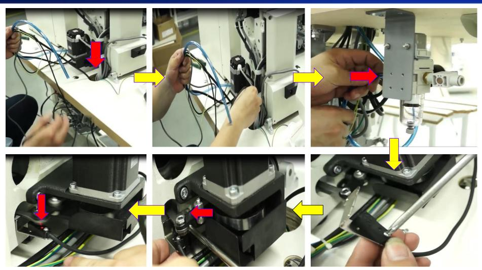
Following above way to do cable threading, then install black sensor as above demo showing ,black sensor is to detect thread trimming movement ,thus ,should be installed under thread trimming level bar to detect level bar each movement then to control button feeding & sewing process .
