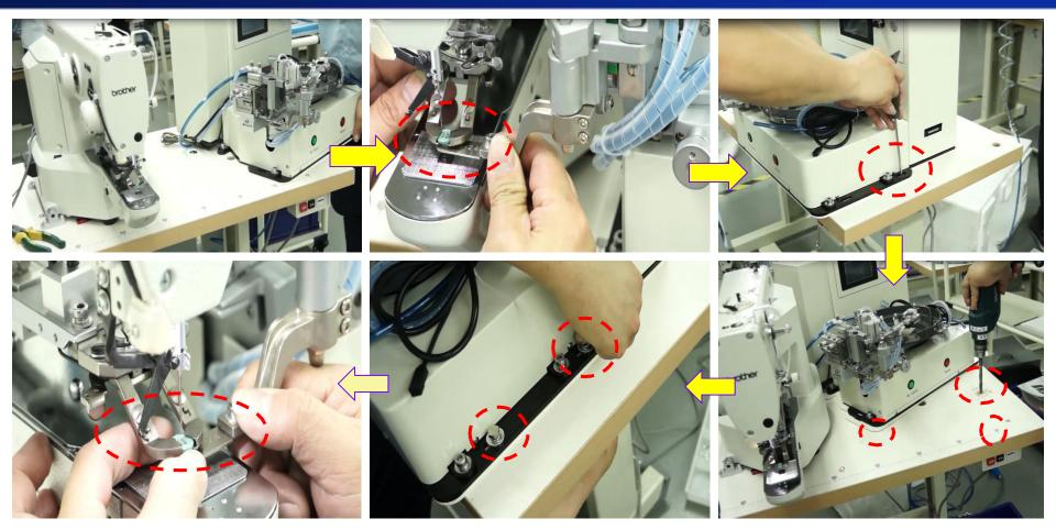
Follow above yellow arrow showing sequence to set button feeder position with machine head, allowed button feeder position difference should be within
