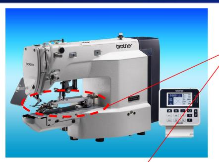
Rmove brother original button clamp and replace it with IMB button clamp
