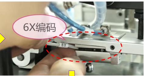
Connect air pipe Y5A, Y5B to desired cylinder as upper left picture shown. Fix sensor X6 to button clamp cylinder with screw as upper right picture shown.
