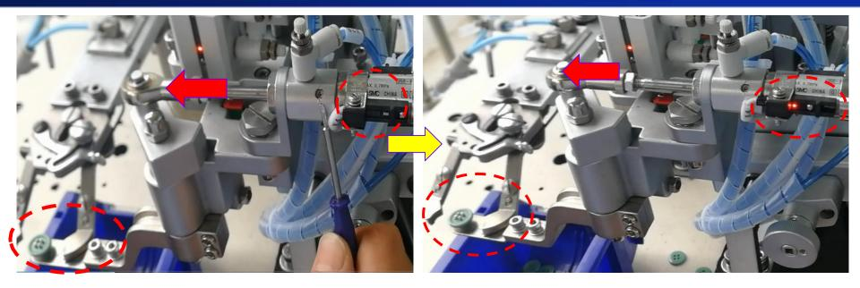
Sensor X4: is to deliver button to button clamp center, when this cylinder pin in most out position sensor X4 light should be ON, if sensor light not in on status, button claw won't reture back for next feeding cycle, button claw will be stuck in button clamp position
