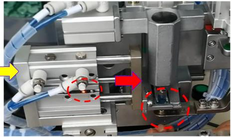
Sensor X7: to limit button out stroke position so that button will not go outside more then drop down.
