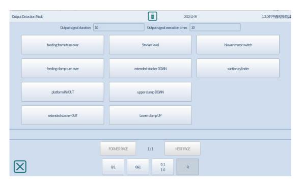
The content of output signal can be customized, and the type of output signal and the parameter setting on the top can be controlled through the bottom
