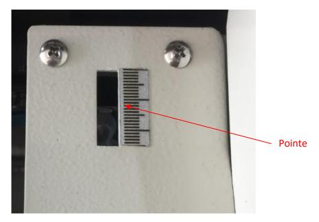
When the buttonhole position is upward, rotate the handle anticlockwise and move the pointer upward to lower the buttonhole position.
