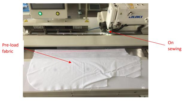
When the "in sewing fabric" is finished, the "pre load fabric" enters the sewing area for sewing. Repeat in turn.
