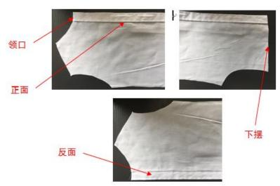
The fabric is evenly spread on the pre laying board, the shoulder of men's cloth piece is facing right, the front is facing up, and the neckline is aligned with the mark at the mark position, as shown in the following figure:
