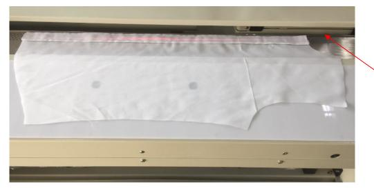
The neckline of the women's cloth piece is placed to the left, facing up, and the neckline is aligned with the mark of the mark position, as shown in the following
