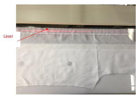
(3) After the fabric is adjusted, release the knee rest switch, and the program will perform automatic sewing.
