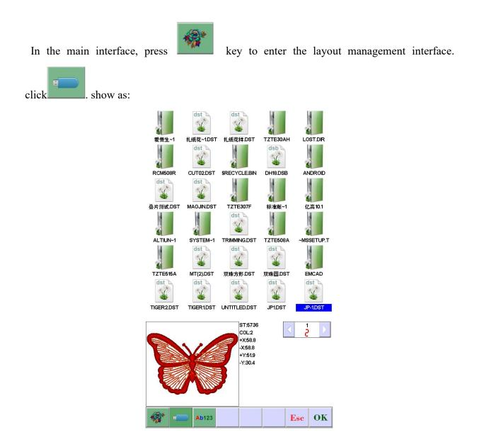
Click the required designs. click OK. automatically display "input process" situation: memory No. And input process. after finishing. automatically return back U disk interface. do the next operation.
