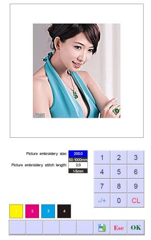
According to the need to set the picture width (height by proportional automatic adjustment), set embroidery needle length, needle step the smaller embroidery reduction degree, the more flower version of the needle will be more, customers can adjust according to
