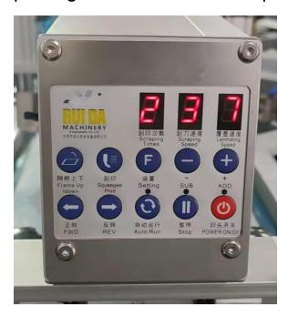
B1: Screen frame up and down: process: when in manual mode, click Pause - Print head switch (on) - Screen frame up and down, click the first lower screen frame up and down button, the screen frame will automatically drop, and click the second lower screen frame up and down button, the screen frame will rise.
